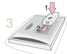
Insert the battery pack down into the battery pack holder (1), then slide it left (2).
